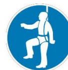
Harness for working at heights, when there are no other collective protection measures in place
